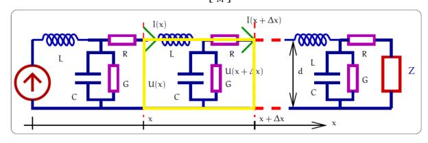
$$0 = U(x + \Delta x) - U(x) + L\Delta x \frac{\partial I(x, t)}{\partial t} + R\Delta x I,$$
